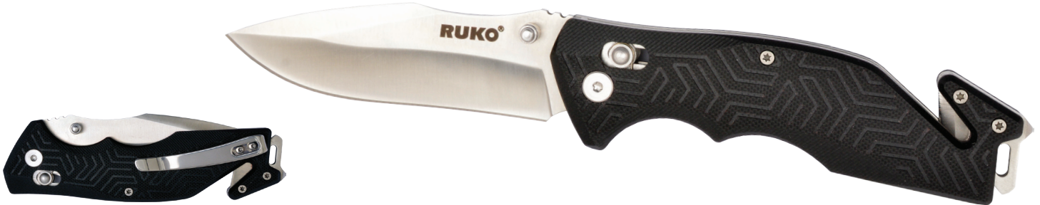
RUK0188BK: glass fiber reinforced nylon handle rescue folding knife, 420A stainless blade, crosslock design, thumb stud opening with low profile pocket clip, seat belt cutting blade, window breaker tip, blade: 3-1/2" closed: 4-3/4" boxed RUK0188BK-CS: as above in clamshell
