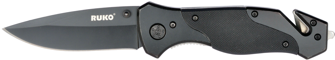
RUK0120: G10/stainless steel handle rescue folding knife, 440A oxide treated blade, locking liner design, ambidextrous thumb stud and low profile pocket clip, seat belt cutting blade, window breaker tip, blade: 3-3/8" closed: 4-3/4", boxed RUK0120-CS: as above in clamshell packaging
