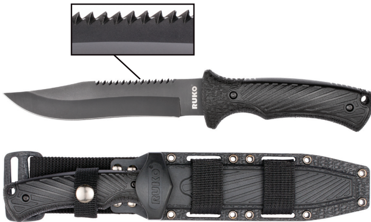
RUK0099: survival knife, 440A stainless black titanium nitride coated ATB saw back blade; 3.5mm rat tail tang blank; non-slip glass fiber reinforced nylon and rubber handle; GFR nylon sheath with web nylon frog and hook & loop straps, D-ring ; blade: 6-1/4" overall length: 11-1/2"
